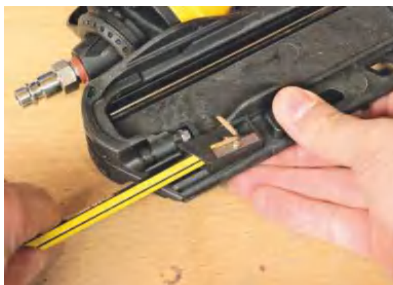
Each gun has its own built-in pencil sharpener!
